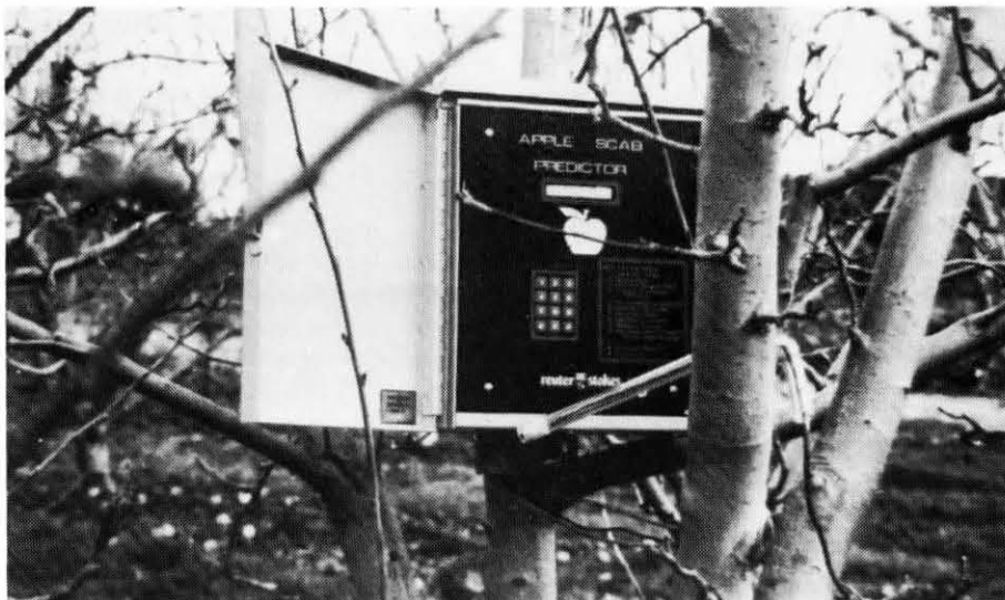
Figure 2. The 'Apple Scab Predictor' provides information on weather conditions favourable for infection.
